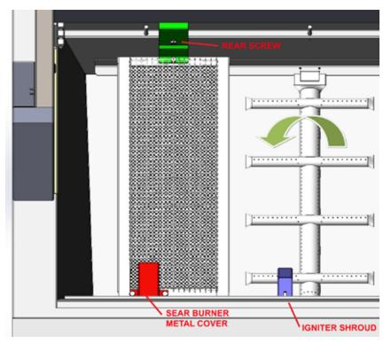
2. Beginning with the Infrared Burner in the upper canopy area of the grill, access the spud orifice shown in the image below. Disconnect the flex hose first. Then use a wrench to hold the brass elbow steady, while using another wrench to remove the lock-nut. You may now remove the elbow out of the burner bracket. Try not to disturb the flex hose connection by unduly bending it too much. Be careful not to damage the wires and copper thermocouple tube nearby.
