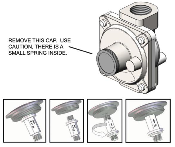
THERE IS A SMALL PLASTIC SPRING GUIDE (USUALLY COLORED BLUE) UNDER THE CAP. UNSCREW THIS PART AND FLIP OVER AND RE-INSTALL IN THE CAP. THEN RE-INSTALL THE CAP INTO THE REGULATOR.
