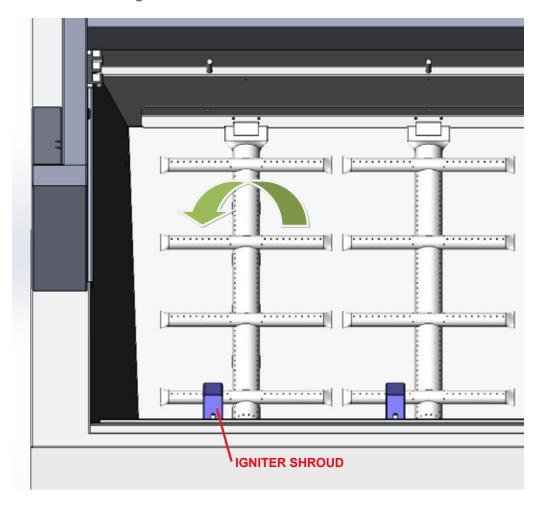
2. Adjust the shroud down onto the burner so it hugs the cross tube / channel as close as possible, but not so far that the burner will not lay flat on the burner hanger at the back of the firebox. Tighten the screws on either side of the shroud.
